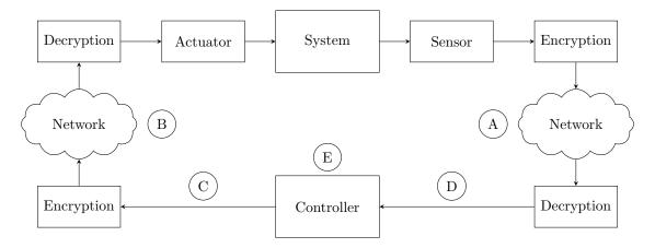
Figure 1: The schematic diagram of a networked control system with encryption-decryption units.
