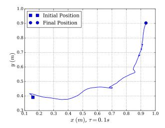
Figure 4: The trajectory of the centre of mass of the robot. The experiment is assumed to be complete when  $||x[k] - x_d|| \le 0.05$ .
