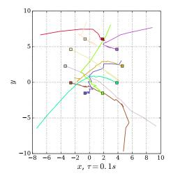
Figure 5: The trajectories of the agents converging to a formation shape under semi-homomorphic encryption information passing.
