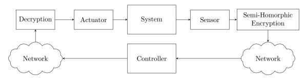
Figure 2: The schematic diagram of a networked control system with semi-homomorphic encryption-decryption units.
