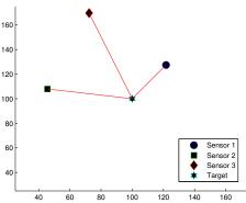
Fig. 2. This figure illustrates two scenarios obtained from each other by reflecting a particular sensor about the emitter position. This reflection does not affect the optimality of the sensor-target configuration.
