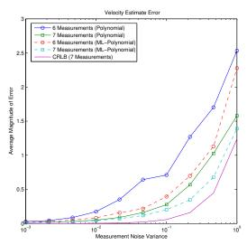
Fig. 4. The error in the estimate of the position and the velocity of the target using the proposed polynomial optimization method (Polynomial) and maximum likelihood initialized at the solution of the optimization problem (ML-Polynomial) after repeating the scenario 100 times with variable noise variances when six and seven sensors are used.
